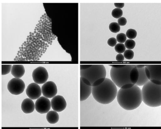
Figure 1. TEM images of silica nanoparticles SiINP003 produced by Stöber synthesis
