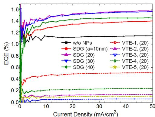
Figure 2.  $EQE$ - $J$  characteristics of the OLEDs without Au NPs, with the Au NP layer fabricated using the SDG-ESP with different values of  $d$ , and with the Au NP layer introduced at  $d = 20$  nm fabricated using VTE with different deposition rates and thicknesses.
