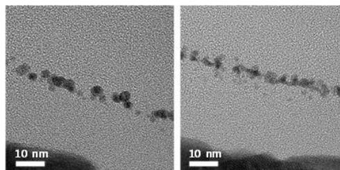
Figure 1. Cross-sectional TEM images of the OLEDs incorporating the Au NPs fabricated using the SDG-ESP (left) and VTE (right).
