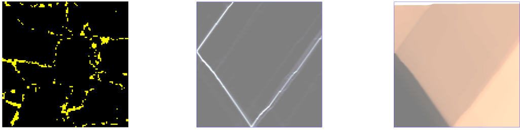
Figure 2: Image CT1 (left), the corresponding failure zones (middle) and kinematic field (right).
