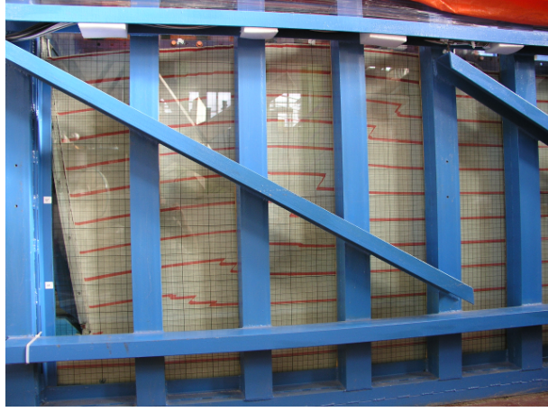
Figure 1: The view on the stand and on the deformed specimen with the evolved slip surface.
