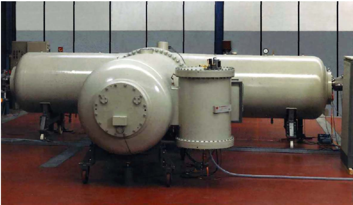
Figure 2.1: The view of the Tandetron 4130 MC T-shaped tank. Ref. [8].
