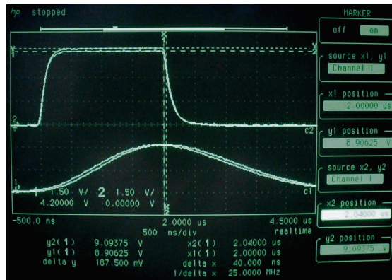
Figure 4.23: The TAC and the amplifier output signal matching. The time difference between the signals arrival to ADCs is minimized by setting the TAC output delay.
