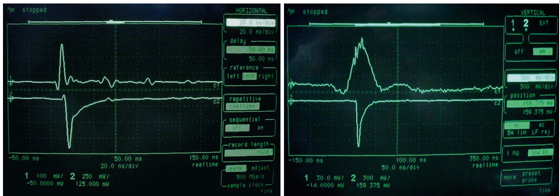
Figure 4.20: The CFD signals. Left: The CFD bipolar and associated output signal converted from the input time detector signal. Right: The CFD bipolar and associated output signal converted from the input energy detector preamplifier timing signal.
