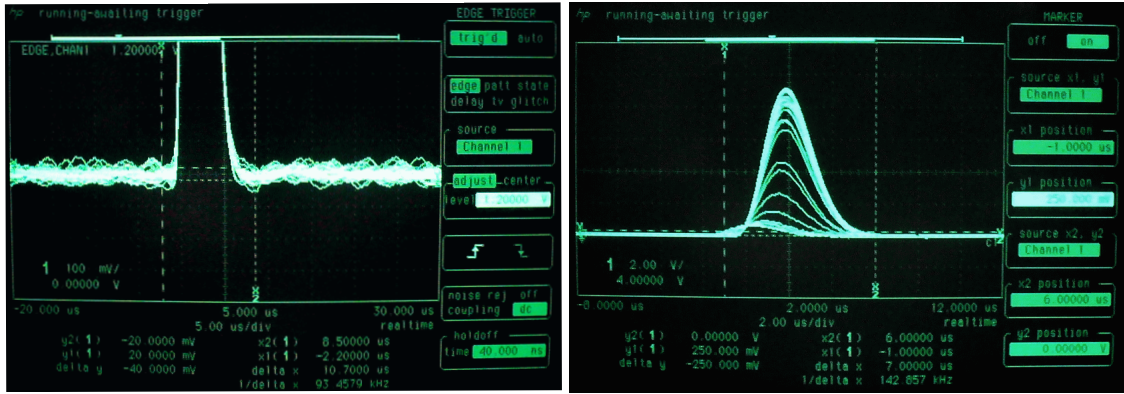
Figure 4.22: The energy detector amplifier tuning. Left: The proper pole-zero cancellation adjustment. Right: The ^{241}\text{Am} \alpha -particle energy unipolar output signals (shaping time 2\ \mu\text{s} ).
