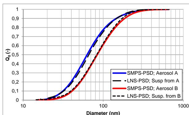
Figure 1: LNS-PSDs of SiO<sub>2</sub> nanoparticles in liquid suspension with the SMPS-PSDs of the corresponding aerosols before precipitation.
