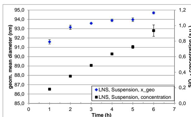
Figure 2: Progression of geom. mean diameter and particle concentration over time, during precipitation in the WESP.
