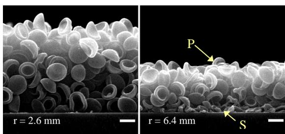
Figure 1. Cross section views by SEM of an ethyl cellulose granular film at different radial locations, collected at 10% RH. Scale bar 1  $\mu$ m.
