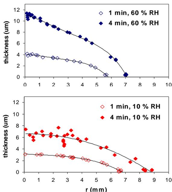
Figure 2. Thickness radial profiles of deposited ethyl cellulose films at fixed inter-electrode separation.
