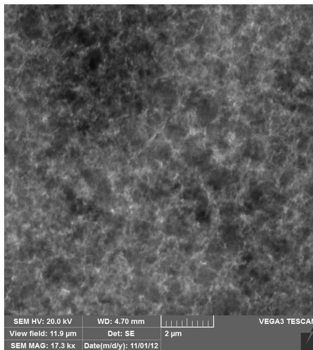
Figure 1. SEM image of NP's generated by evaporation/condensation of metallic Pb at  $T_R=860$  °C,  $Q_R=1000$  cm<sup>3</sup>/min.
