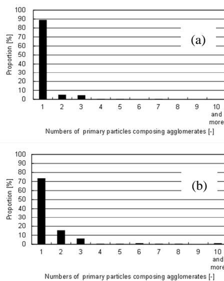
Fig. 2 Distributions of the number of primary silica particles composing the respective agglomerates after the collisions
