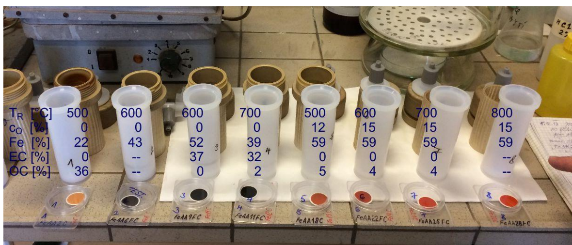
Fig. 2: Concentrations of Fe, EC and OC of the samples prepared by pyrolysis and oxidation of FeAA3 in dependence on T_R .
