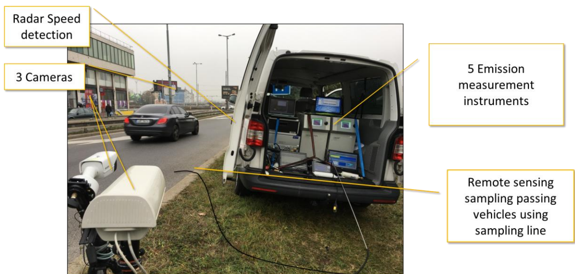
Fig. 1: Pre-selection of passing vehicles using remote sensing – exhaust plume roadside sampling
