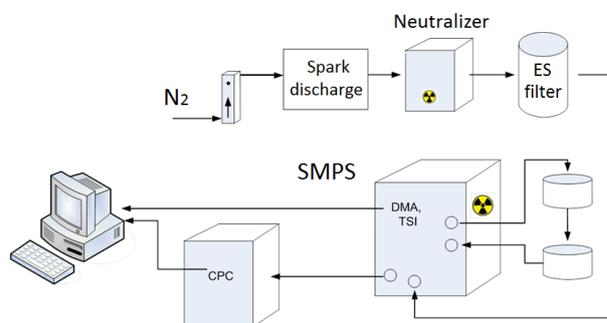
Figure 2. Experimental set-up used to measure the capturing efficiency shown in figure 1.
