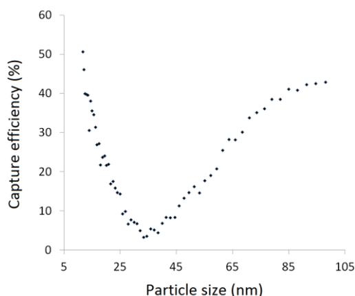
Figure 1. Capturing efficiency of aerosol nanoparticles by an ES filter.
