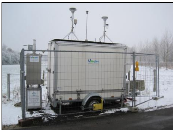
Figure 1 One of the mobile instrument vans placed downwind with a Leckel alongside (left).
