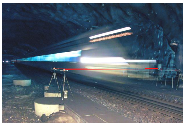
Figure 1. Train detection system at Arlanda Central (red beams illustrating infrared light).
