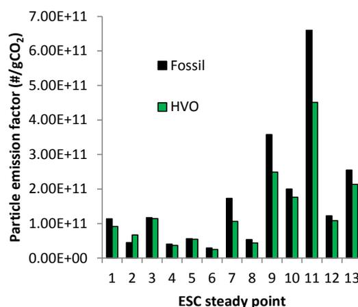
Figure 1. Solid particle engine-out number emission factors with a fossil diesel fuel and hydrotreated vegetable oil (HVO) at different ESC cycle steady test points. Particle concentrations were measured with the ELPI behind the DED sampling
