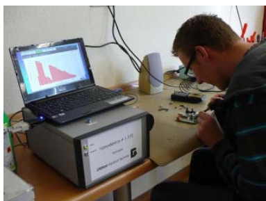
Figure 2: Measurements at workplaces, determination of all particles caused by soldering
