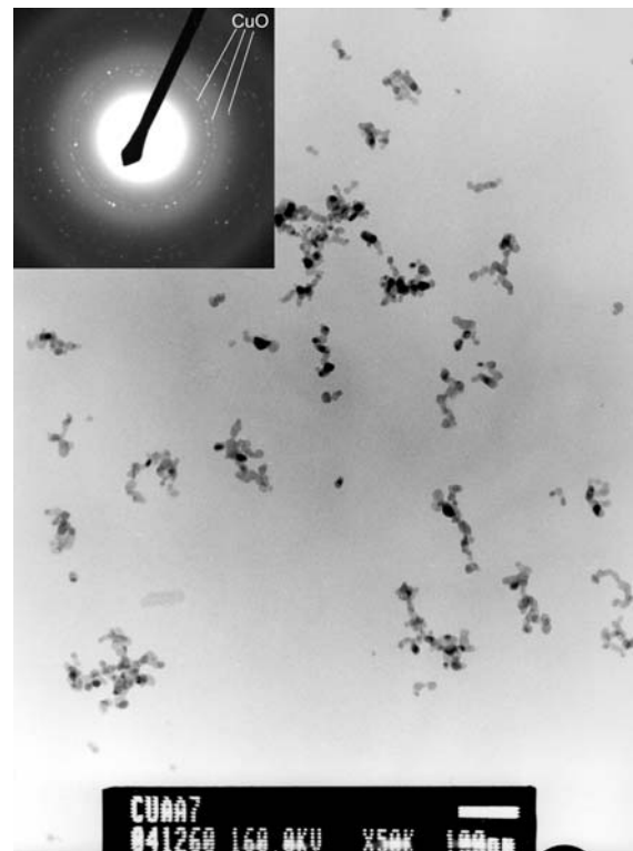
Fig. 7 Bright field TEM image and SAED pattern of the sample CuAA7. T_R=500^\circ\text{C} , T_S=160^\circ\text{C} , Q_R=600\text{ cm}^3/\text{min} , oxidation.
