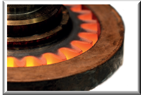
Induction heat treatment for a gear
