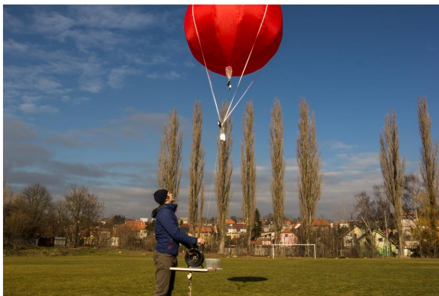
Fig. 1: Temperature and humidity vertical profiling, Kladno-Švermov, 6. 2. 2016
