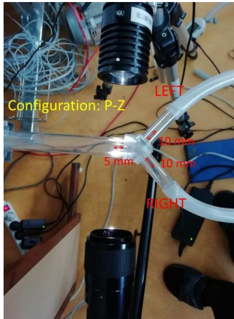
Fig. 1: Positions of measuring points upstream and downstream of the replica of the first bifurcation in the human airways.
