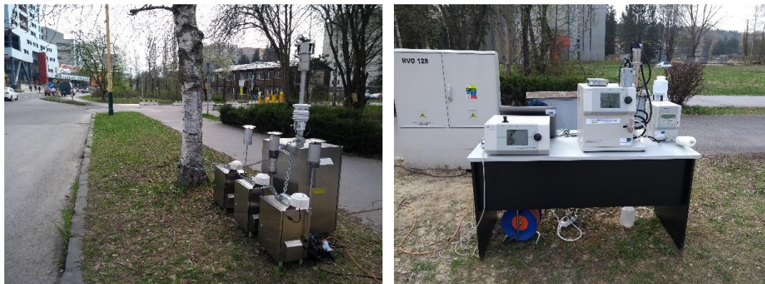
Fig. 1: Measurement devices Leckel LVS3—3x and Fidas 200S ( left ) and SMPS and APS ( right ).
