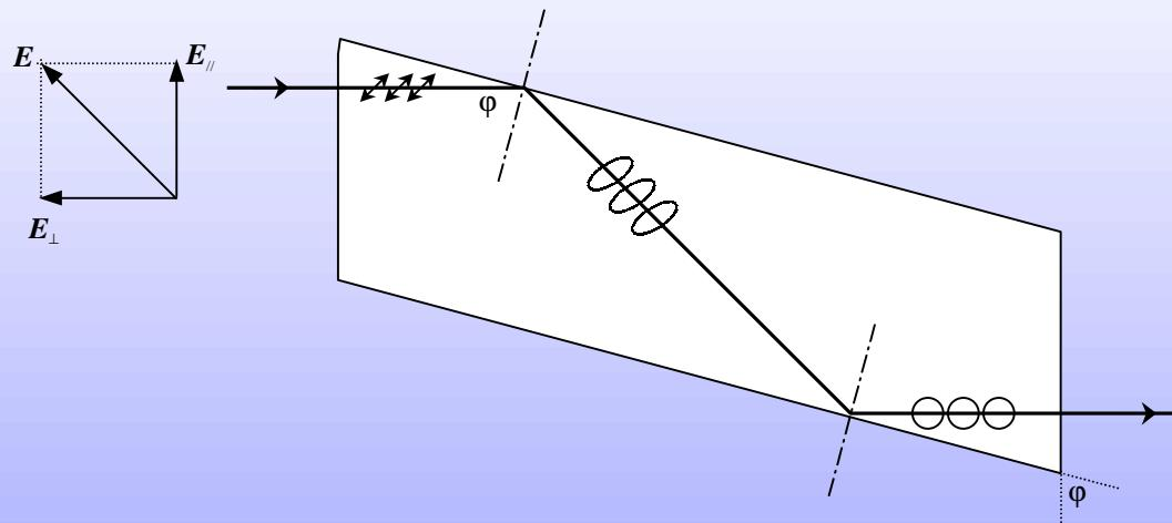
Combination of 2 Fresnel prisms: half-wave plate
