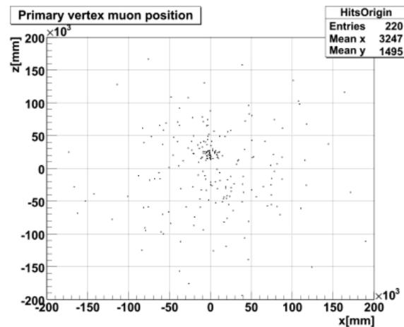
Figure: Initial  $XZ$  positions of muons eventually hitting the detector. Generated from  $400 \times 400$  m surface.
