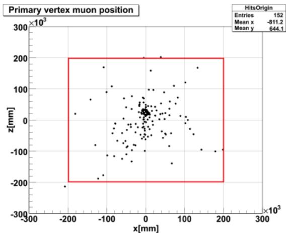
Figure: Initial  $XZ$  positions of muons eventually hitting the detector. Generated from  $600 \times 600$  m surface.
