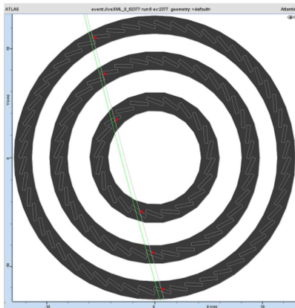
**Figure:** Example of a cosmic track with hits in all barrel layers of the Pixel Detector
