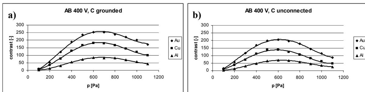
**Figure 2.** Dependences of the contrast on the pressure of water vapors in the specimen chamber. Segments A and B are at the potential of 400 V, segment C is a) grounded or b) unconnected.
