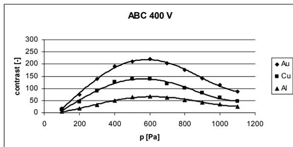
**Figure 3.** Dependences of the contrast on the pressure of water vapors in the specimen chamber. Segments A, B and C are at the potential of 400 V.
