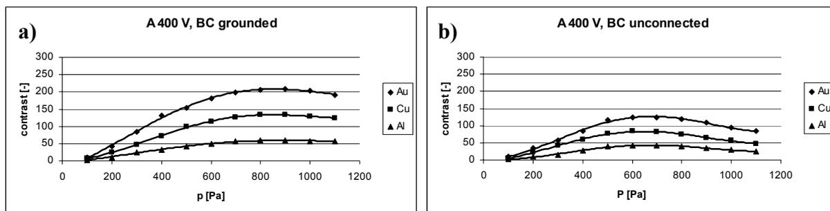
**Figure 1.** Dependences of the contrast on the pressure of water vapors in the specimen chamber. Segment A is at the potential of 400 V, segments B and C are a) grounded or b) unconnected.
