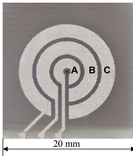
**Figure 4.** Segmental ionization detector with the concentric segments A, B, C.
