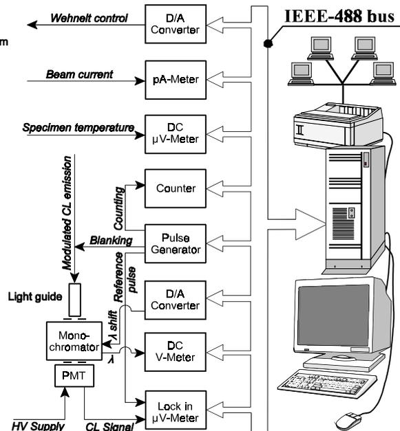
**Fig. 2.** IEEE-488 bus layout for the control of the CL emission spectra measurement.
