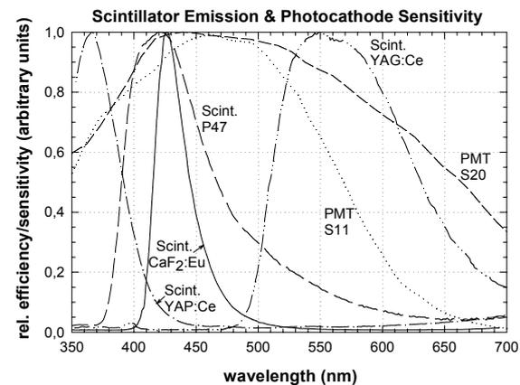
**Fig. 3.** Normalized CL emission spectra and spectral sensitivities of some scintillators and PMT photocathodes, respectively.
