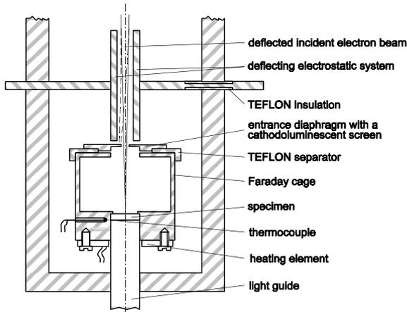
**Fig. 1.** Specimen chamber arrangement of the CL experimental equipment.
