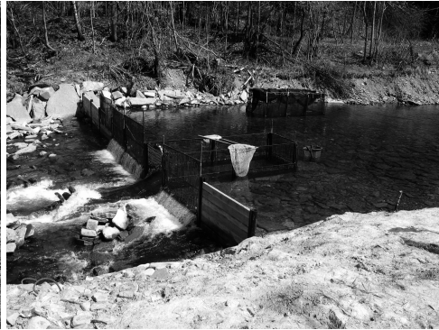
Fig. 2. The constructed trap was used for the monitoring of spawning migration of brown trout in the tributary of Morávka reservoir, a) the concrete board on the stream bottom, b) the assembled trap.
