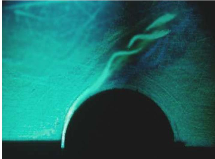
**Fig. 22** Coanda-effect attachment of propane-butane wall jet issuing into air at a quite low Reynolds number – the clearly discernible : Taylor-Görtler instability vortices are visualised by Töpler's schlieren method.
