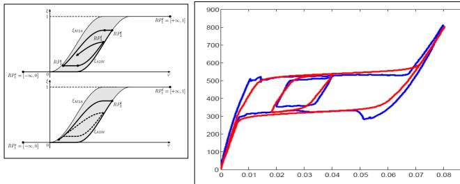
Stress strain curve for a NiTi wire. The blue curve shows the real, experimentally obtained behaviour, the red one the model developed at LUM.
