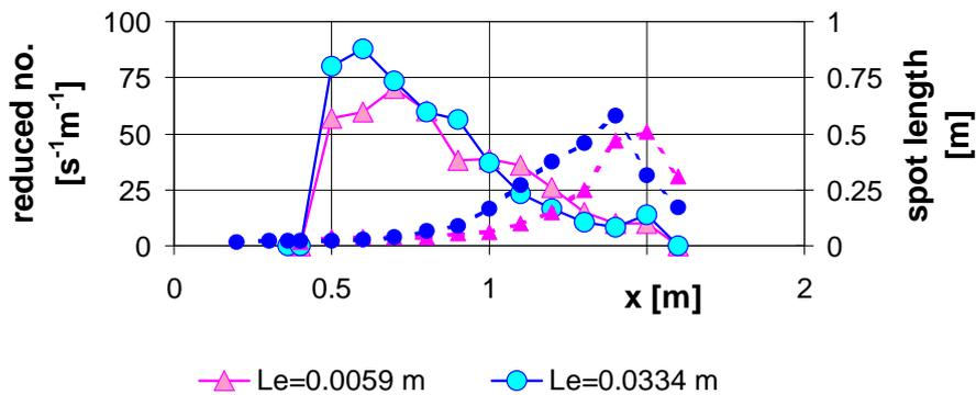
Figure 11 Distribution of reduced number (light colour) and mean length of the identified turbulent regions (bright colour) versus the distance  $x$ .
