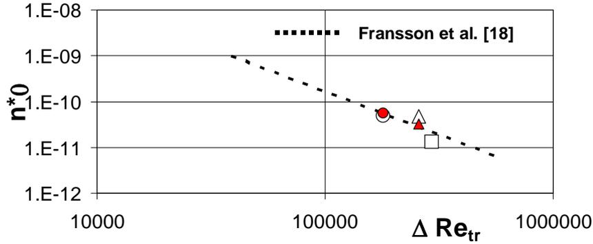
Figure 7 Dimensionless spot production rate as function of the transitional region length  $Re$  (marks as in Fig. 6, filled marks are calculated from the wavelet analysis).
