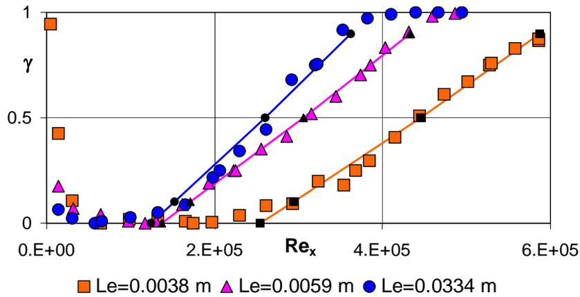
Figure 5 Transitional intermittency factor as function of the local Reynolds number.
