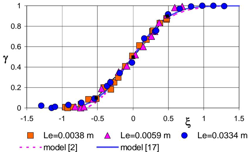
Figure 6 Universal intermittency function: models according to [2] and [17] and experimental data.
