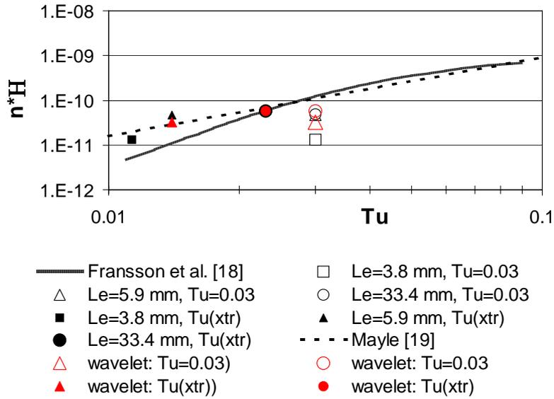
Figure 8 The dimensionless spot production rates plotted versus turbulence level  $Tu$  (in the leading edge plane  $x = 0$ ,  $Tu = 0.03$ , empty black marks and in sections of the transition start  $x = x_{tr}$ ,  $Tu < 0.03$ , filled marks).
