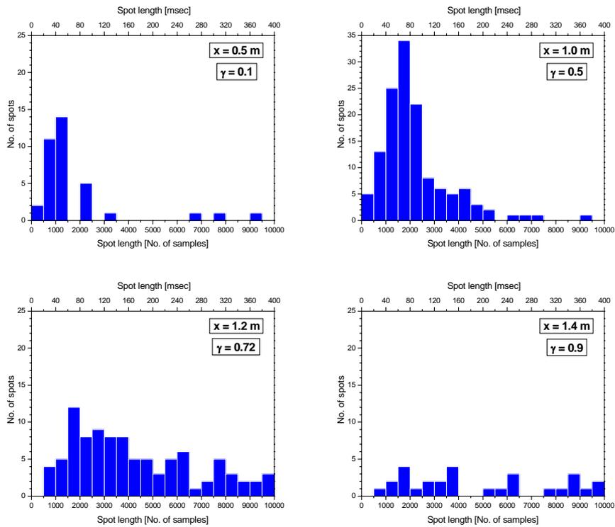
Fig. 9. Number of spots as a function of spot length (for the coordinates  $x = 0.5, 1.0, 1.2$  and  $1.4$  m), GT1,  $Le = 5.9$  mm.
