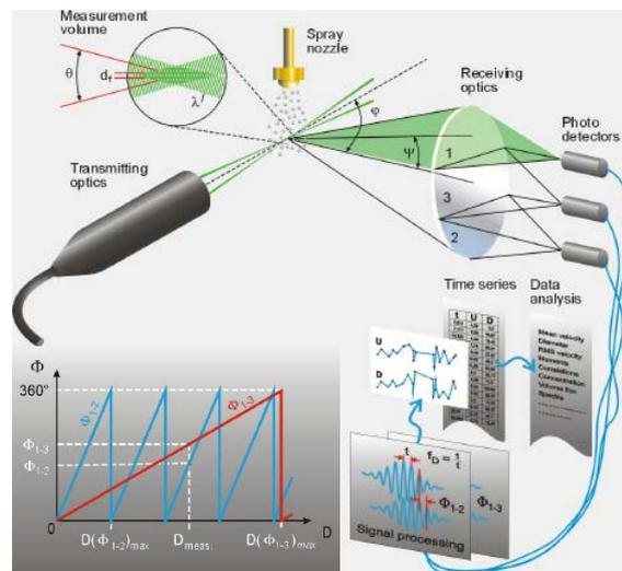
Fig. 4 PDA system principle
