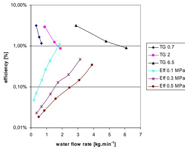
Fig. 7 Atomization efficiency against flow rates
