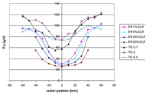
Fig. 5  $D_{20}$  distributions in the spray cone
