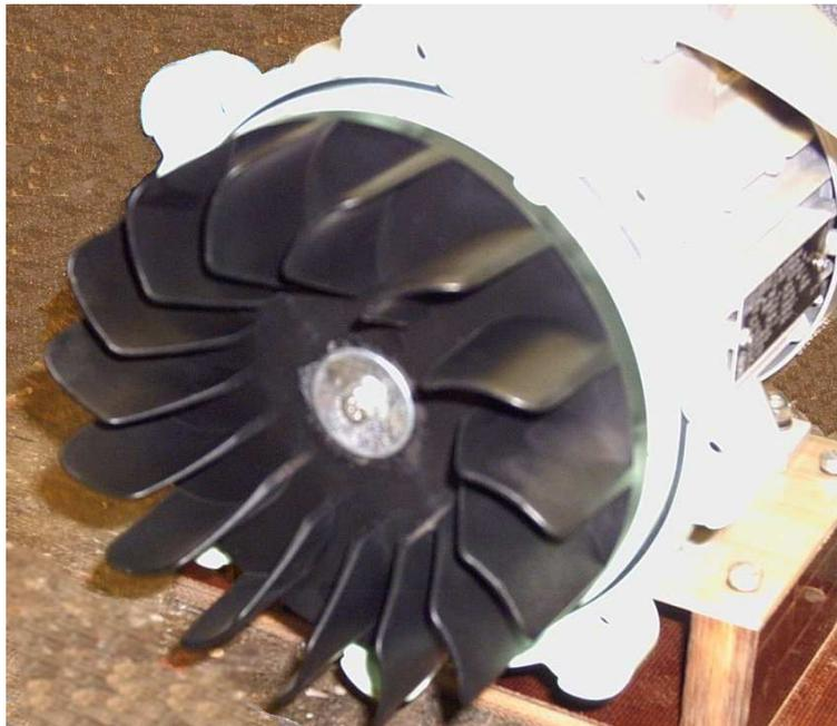
**Figure 4** Photograph of the rotor of the investigated blower (taken by Mr. J. Šafář). Note the absence of the rotor cover disk. The essential geometric parameters (as defined in ref. [2]) are as follows: rotor outer diameter:  $d_Y = 147$  mm, blade exit length  $b_Y = 39.7$  mm. Calculated from these values, the exit area is  $F_Y = 18.334 \cdot 10^{-3} \text{ m}^2$ .
