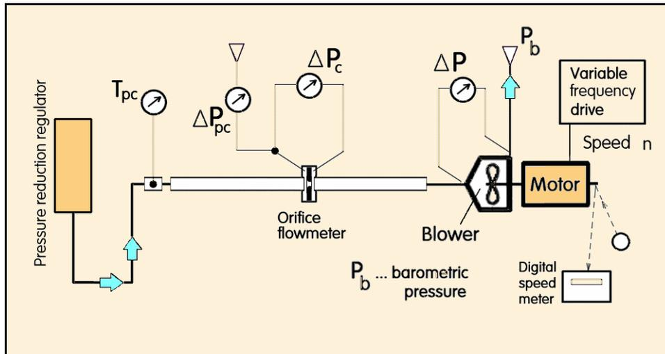
**Figure 5** Schematic representation of the performed experiments. The air flow rate is dictated by the external source. While the speed of the driving motor is kept constant, the air flow supplied from the regulator is gradually increased and measured by the orifice flowmeter.
