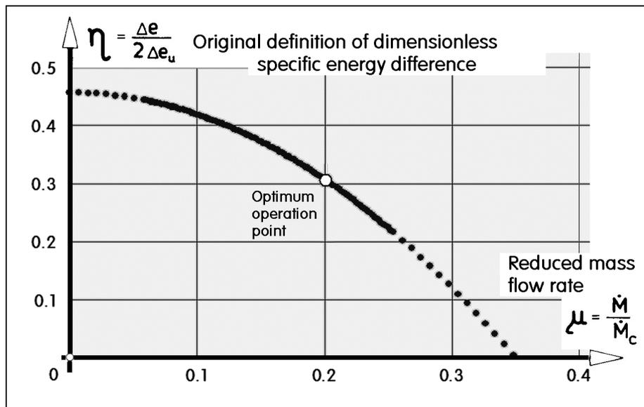
**Figure 12** The dimensionless co-ordinates  $\mu$  and  $\eta$  for universal characterisation of blower behaviour at any rotational speed - as originally recommended in ref. [2]. The curve and the optimum point shown here are actually valid for a water pump used in that reference as an example.
