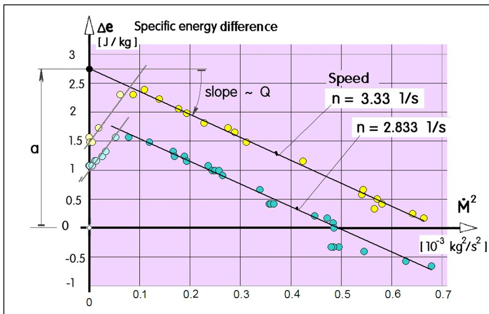
**Figure 10** The two coefficients  $\alpha$  and  $Q$  that define the blower behaviour conforming to the quadratic model were evaluated from the experimental data by plotting the specific energy difference against the *square* of the mass flow rate – this transformation of the diagram should convert the dependences described by eq. (3) into straight lines, which is here seen to be indeed the case.
