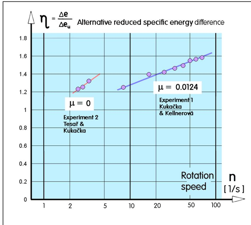
**Figure 14** The decrease of the stalled flow region with increasing Reynolds numbers (no doubt due to the less tendency to separation in flows with turbulence) was found in the experimental data and is documented here by the measured data showing an increase of the relative specific energy difference with increasing rotational speed at very small relative output flows.
