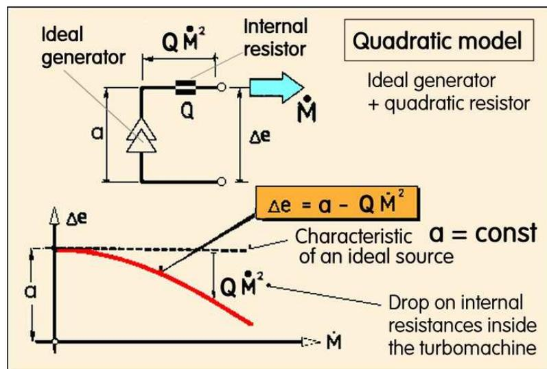
**Figure 2** The quadratic model of the blower behaviour. The model explaining the usually encountered decrease of the available specific energy at the blower exit with increasing delivered mass flow rate is based on an imagined series connection of an ideal generator, which would exhibit a simple horizontal line characteristic, and a quadratic restrictor.
