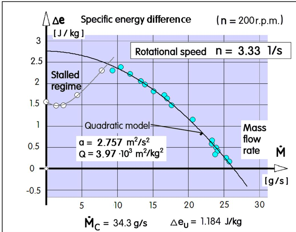
**Figure 9** Yet another set of experimental data for the loading characteristic of the blower was obtained at another, higher still rotational speed. The relative extent of the stalled regime (where the symbols are empty, white) decreases as the motor speed is increased and this phenomenon becomes less prominent as the speed is increased.
