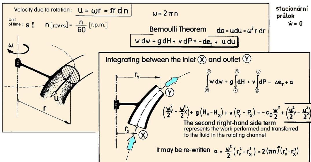
**Figure 3** (Taken from textbook [2]) the expression for evaluation of the specific work  $a$  in Fig. 2 is obtained very simply by expansion of the Bernoulli Theorem, adding to it the term representing the kinetic energy of the velocity  $u$  of the rotational motion.
