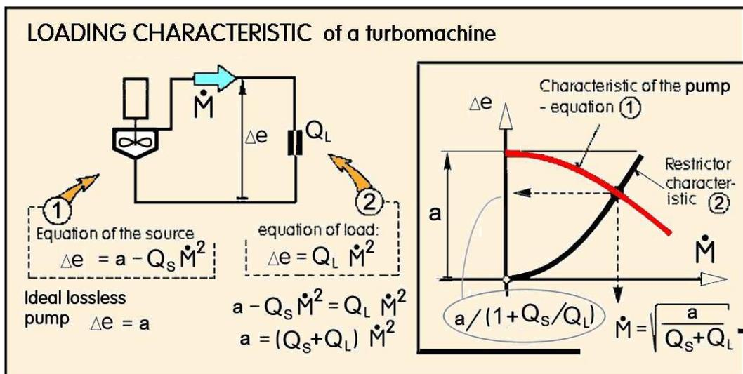
**Figure 1** General idea of evaluating the conditions in an aerodynamic circuit driven by a turbomachine blower by the “black box” approach - by locating the intersections of the characteristics of the blower and of the load. The mathematics of this solution presented here is based on the assumption of purely quadratic behaviour of the blower as well as of the load.
