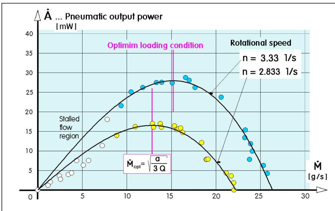
**Figure 11** Power characteristics the measured blower at two different rotational speeds. Values evaluated from the experiments are confronted with the optimum loading predictions resultant from the quadratic model of Fig. 2. Of course, the maxima are flat so that the prediction accuracy is not critical – nevertheless, it is apparent that the quadratic model predictions provide a very good tool for designing fluidic circuits.
