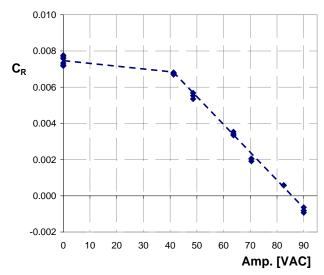
Fig. 16: Airplane rolling moment vs AFC voltage applied to the right wing.  $\alpha$ =2 deg, V=20m/s.
