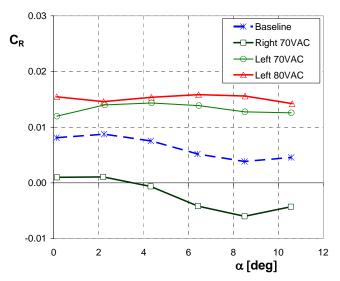
Fig. 15: Rolling moment vs airplane incidence with AFC applied either to the right or left wings. V=20m/s.
