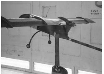
Fig. 12b: The airplane as installed at IAI LSWT.
