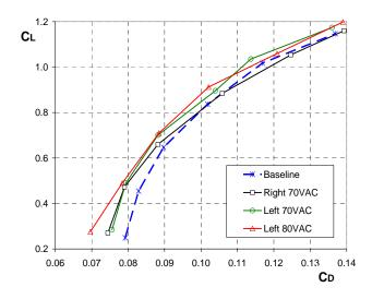
Fig. 13: The baseline lift of the plane, as measured at IAI LSWT, at the Reynolds number range corresponding to 15, 20 and 25m/s. Roughness strip installed.
