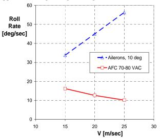
Fig. 18: A comparison between the expected roll rate between 10 deg aileron deflection and AFC induced roll (using 70-80Vac) at V=15-25 m/s flight speed.
