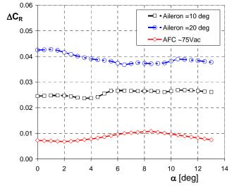
Fig. 17: A comparison of the rolling moment induced by conventional aileron deflections of 10 and 20 deg to activation of the one wing AFC at 70-80 vac (average of two wings) at V=20 m/s.
