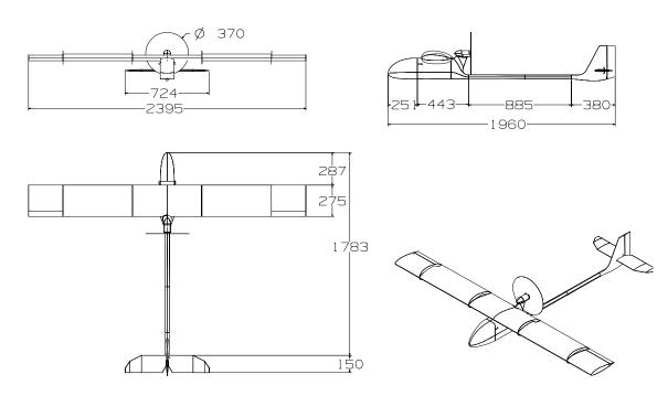
Fig. 10: The configuration of the flight demonstrator. Dimensions in mm. Wing surface 0.66m<sup>2</sup>, wing incidence 3 deg at airplane zero incidence.
