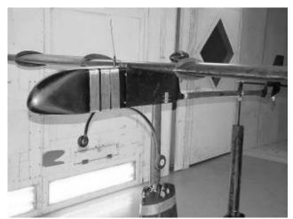
Fig. 12a: The airplane as installed at IAI LSWT.
