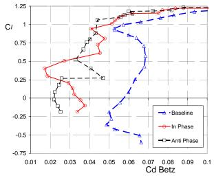
Fig. 5b: The effect of actuation on the lift vs drag. Re=370k, Up=40m/s, forcing all actuators in phase and every other actuator phase inverted. Triangles – baseline.
