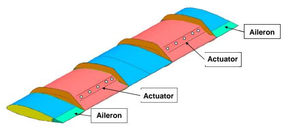
Fig. 11: The layout of the wing. The red sections are the Glauert AFC sections and the blue regions are the conventional airfoils. The conventional ailerons are shown at both wing tips, in green. The middle section and the Glauert sections are 600 mm each. The aileron sections are 300 mm each. The aileron is 20% of the chord. A switch on the remote control was used to alter the joystick purpose, from controlling the aileron deflection to controlling the AFC voltage to either right or left wings.
