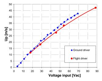
Fig. 4b: Amplitude response of the G275 airfoil actuators at 1380Hz, driven by the ground system (blue diamonds) and by the prototype of the flight drive system (circles). Obtaining about Up=40m/s consumed only about 2 Watts.
