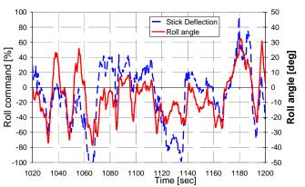
Fig. 20: Flight test data showing the roll command (left side ordinate) and roll angle (right side ordinate) vs time. At 1200>t>1020 sec the roll control was induced *only* via AFC applied to either the right or left wings using the stick deflection.
