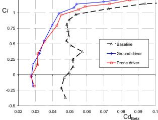
Fig. 7b: Baseline and controlled lift vs incidence at Re=370k operated by the ground and flight drive systems. All actuators operate in unison, 85Vac, Up~45m/s.
