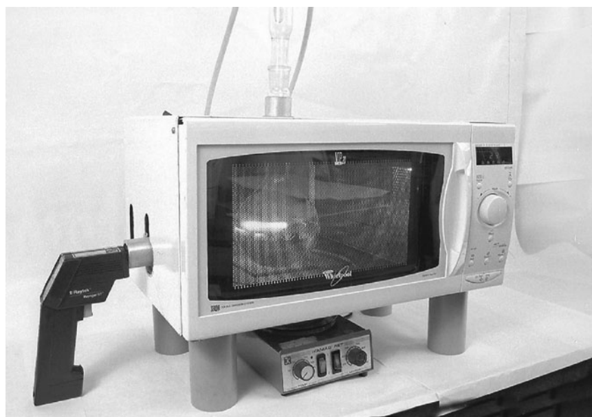
Fig. 19.13. Photochemistry in a microwave oven (the EDL floats on the liquid surface).
