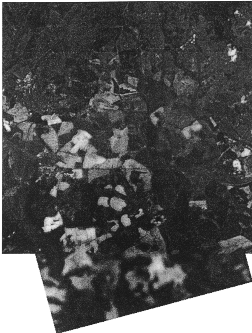
Figure 5. The registered images. Intensity values in the overlapped area are calculated as the mean of the corresponding intensity values of the reference and sensed images.
