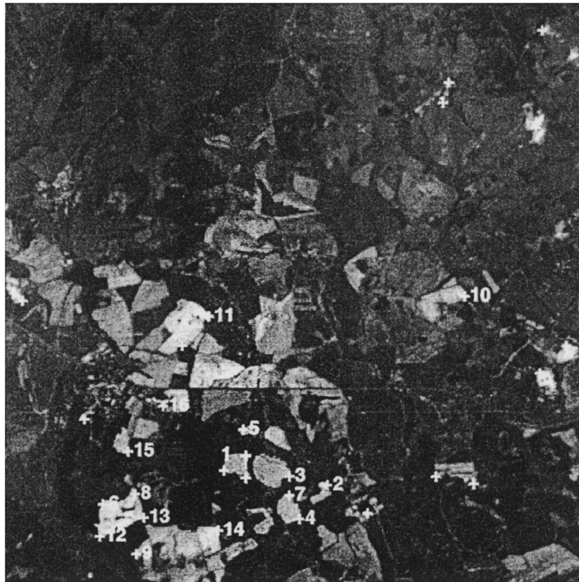
Figure 3. Reference image—SPOT subscene of the size 400 \times 400 pixels—with the detected control point candidates. Numbered CPCs have their counterparts in the sensed image.
