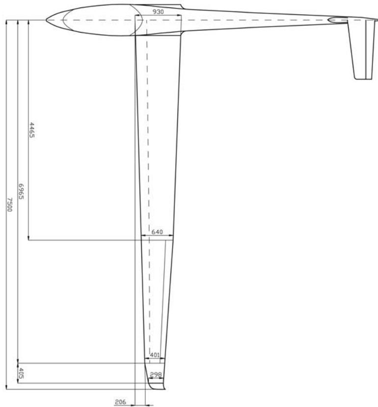
*Fig. 2 Main dimensions of TST10a wing*
