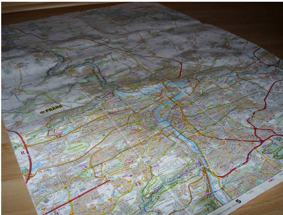
Figure 1.1: Perspective distortion of the image caused by a non-perpendicular view.
