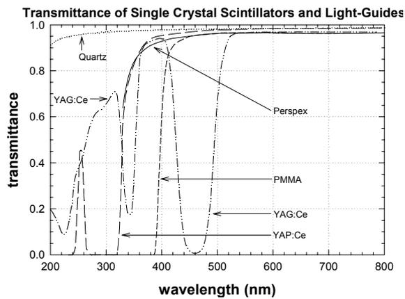
**Figure 2.** Optical transmittance of the YAG:Ce (thickness 0.41 mm) and YAP:Ce (0.37 mm) single crystal scintillators and of the PMMA (50 mm), Perspex (52 mm) and quartz (50 mm) light-guiding materials.
