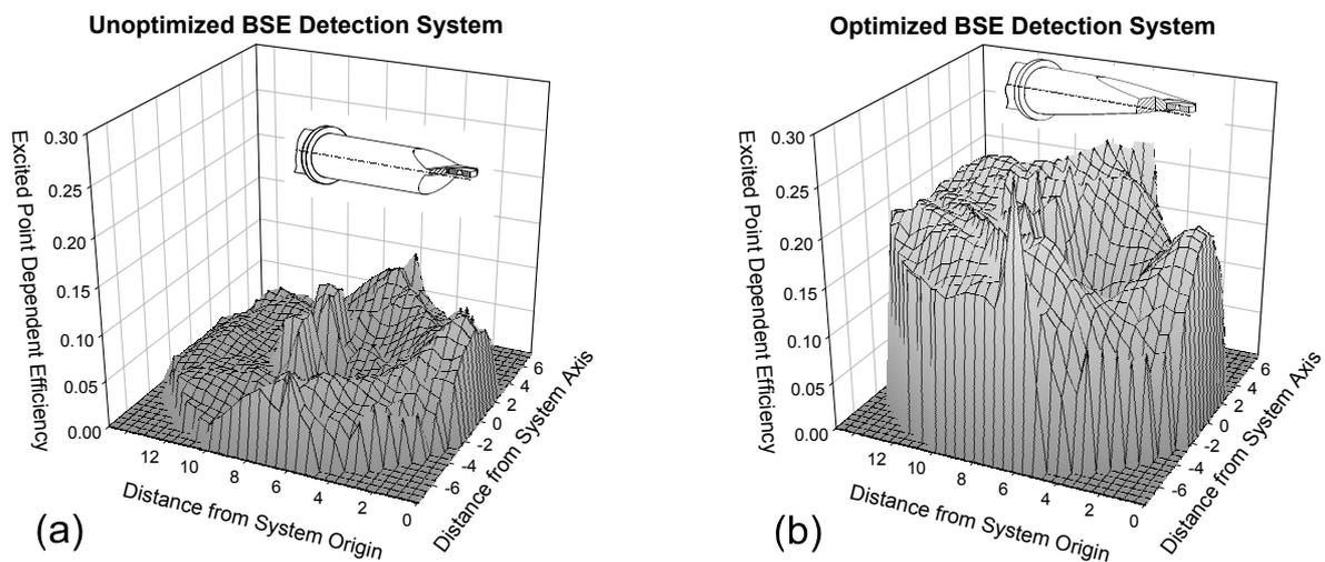
**Figure 3.** Monte Carlo simulation of the efficiencies of the photon transport through whole scintillation detection systems possessing (a) the bad (b) the good geometry. 3D graph represents the dependence of the photon transport efficiency on the coordinates of the excitation point at the surface of the scintillator.
