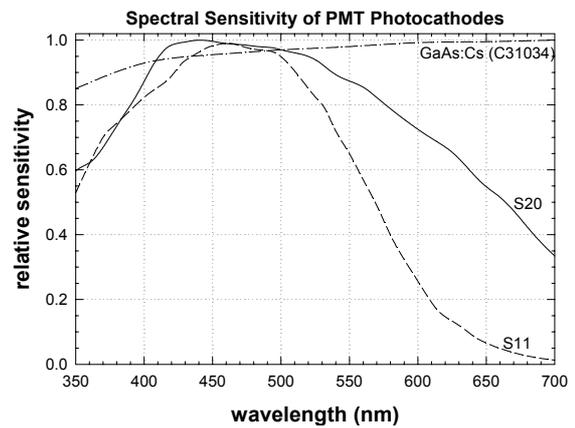
**Figure 1.** Normalized spectral response of the sensitivities of PMT photocathodes. **S20:** THORN EMI 9558B, **S11:** TESLA 65PK415, **GaAs:Cs:** BURLE C31034.
