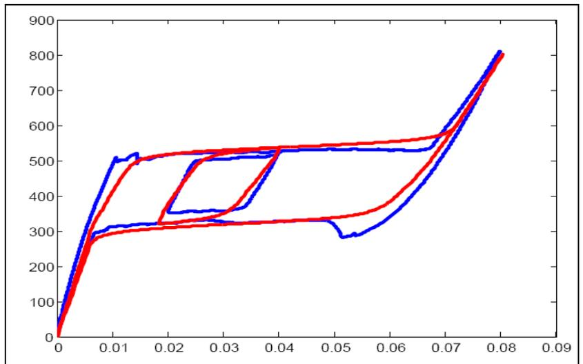
Stress strain curve for a NiTi wire. The blue curve shows the real, experimentally obtained behaviour, the red one the model developed at LUM.
