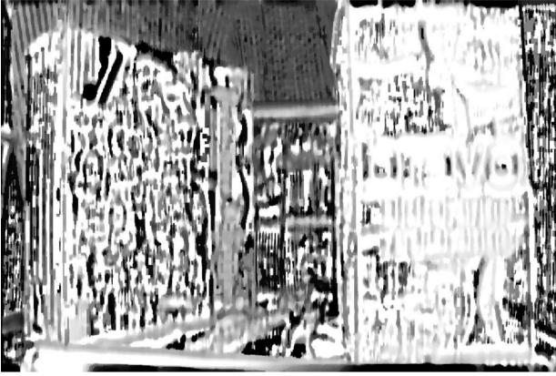
(b) depth map got by auxiliary algorithm (8), error averaged by 7 \times 7 window, depth map finally smoothed by 23 \times 23 median filter
