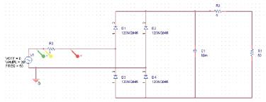
• Capacitive input stage - nonlinear load (PSpice model)
