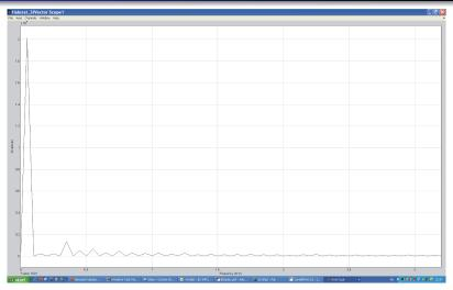
• Spectrum of Voltage at the connection point (UHC ON)
