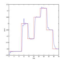
Comparison between the LQ controller and the mixture-based controller.
