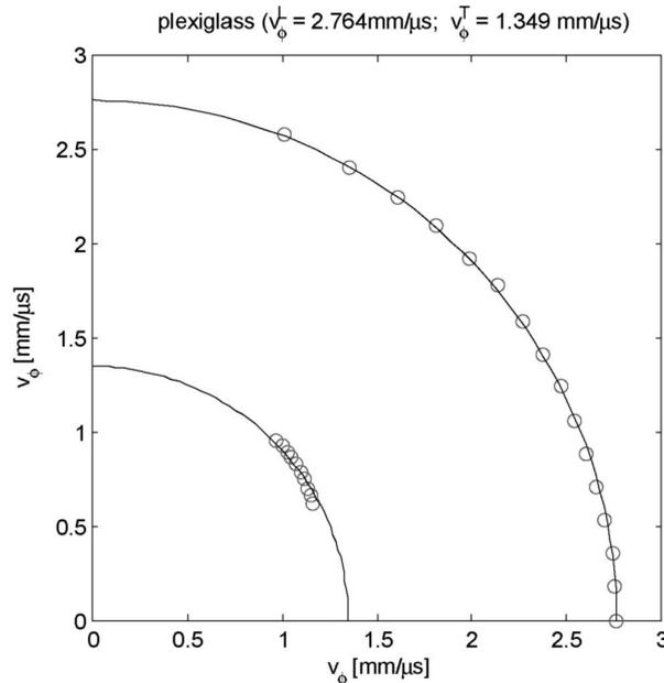
Figure 7: Plots of the phase velocities [mm/μs] propagating through cylindrical specimen. Circles - experimentally obtained data, Solid lines - phase velocities for calculated  $c_{ij}$ .
