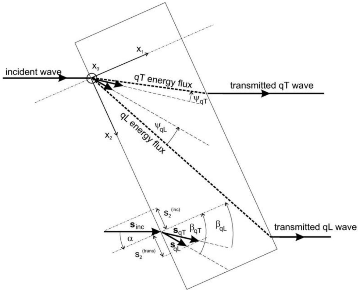
Figure 1: An interaction of a single planar wave with an anisotropic plate-like specimen.
