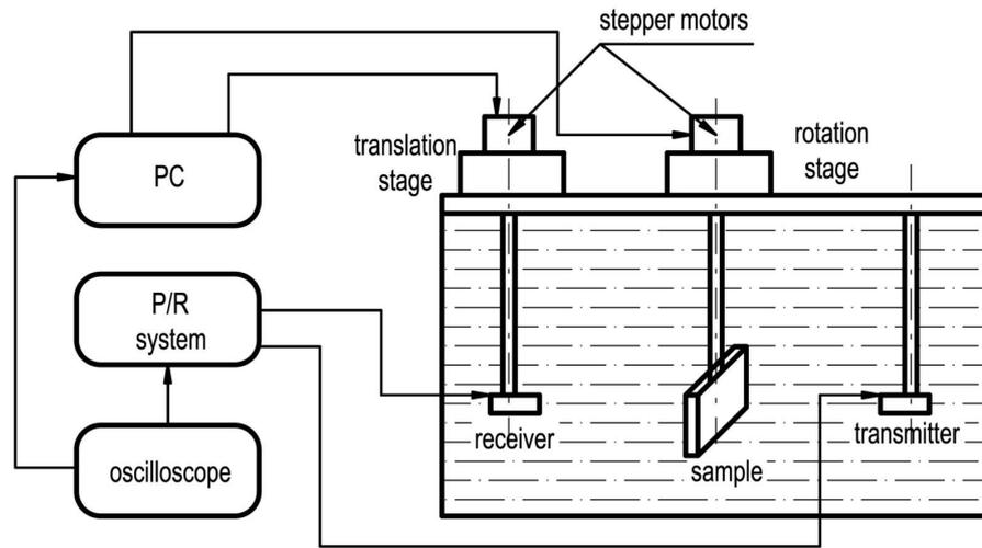
Figure 3: Experimental configuration
