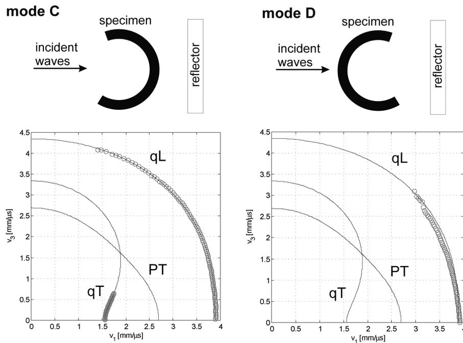
Figure 8: Figure 8: Plots of the phase velocities [mm/ $\mu$ s] propagating through bone specimen. Circles - experimentally obtained data, Solid lines - phase velocities for calculated  $c_{ij}$ . Horizontal axis - phase velocity in  $x_3$  direction (fiber direction), Vertical axis - phase velocity in  $x_1$ .
