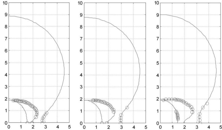
Figure 4: Plots of the phase velocities [mm/ $\mu$ s] propagating in the wave normal directions through CFRP plate specimens of 2, 4 and 8 mm thickness.
