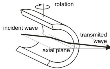
Figure 6: Measurements in an axial plane of a cylindrical specimen.
