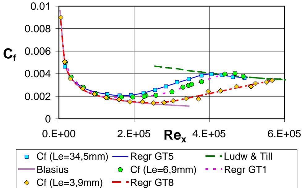
**Figure 4** Distributions of skin friction coefficient in boundary layers (grad  $P = 0$ ) under external grid turbulence flows with the intensity of velocity fluctuations  $I_{u_e} = 3\%$  at the onset of the layer  $x=0$
