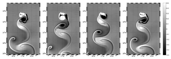
Figure 2. Time varying shedding for 30th, 35th, 40th and 45th model days (from left to right). Colours represent surface vertical vorticity.
