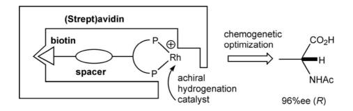
**Scheme.** Artificial metalloenzymes for enantioselective hydrogenation reactions. The host protein (either avidin or streptavidin) displays a high affinity for the biotin anchor. Introduction of a spacer and variation of the ligand scaffold allows to chemically optimize the enantioselectivity. Fine tuning of the selectivity can be achieved via site-directed mutagenesis of the (strept)avidin.
