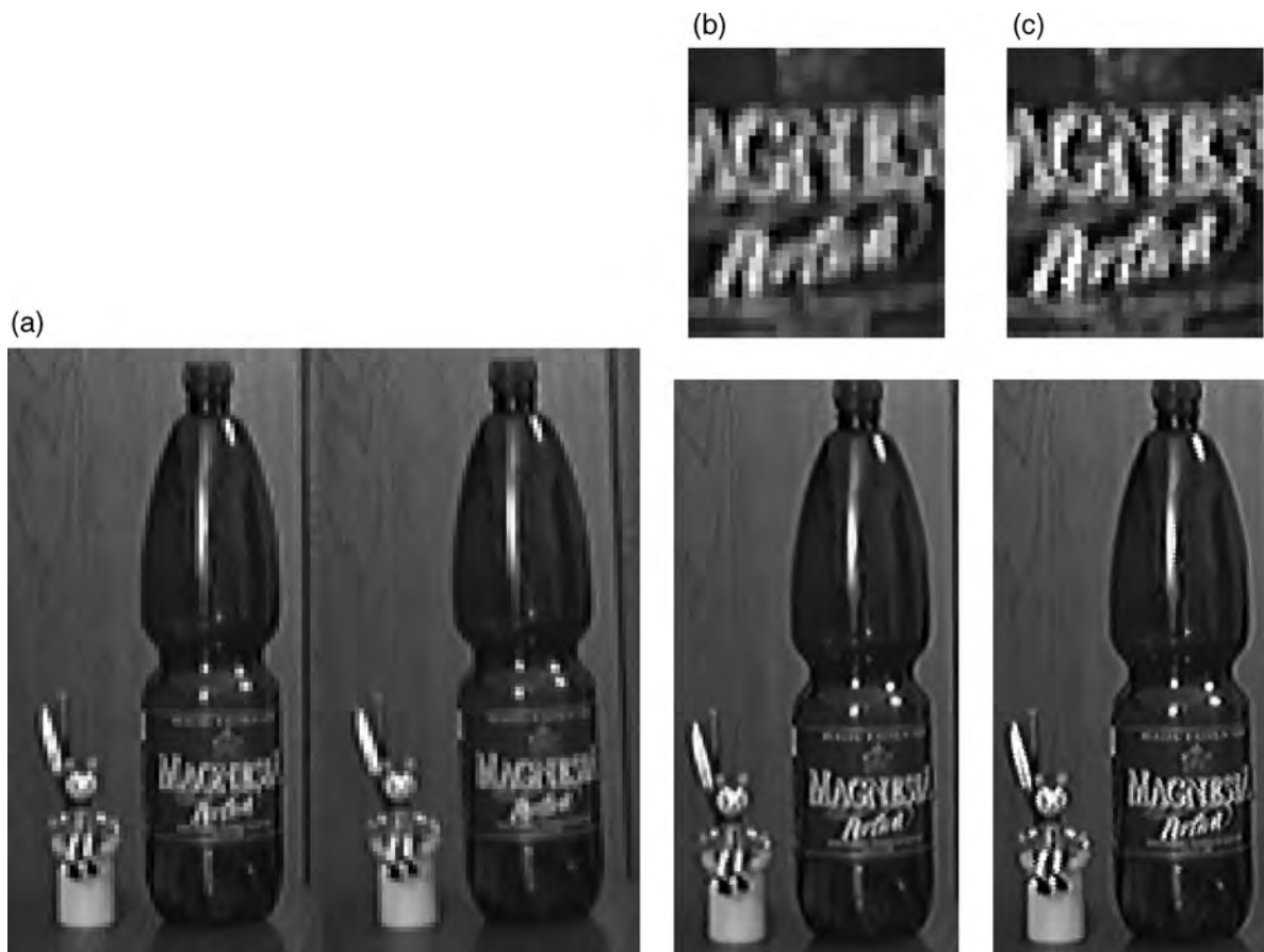
FIGURE 7. SR with registration. Ten frames were extracted from a video sequence recorded by a webcam (exposure time 1/10 s). Two such frames are in (a) printed in the size of output HR images for comparison reasons. Due to slight rotation of the webcam during shooting, registration parameters were first estimated by a registration method. Two approaches were compared: (b) Input frames were registered according to the parameters and BSR was applied on the registered images. (c) The registration parameters were used to modify decimation operators and BSR was applied to the original unregistered images. Better performance of the second approach is apparent from close-ups in the top row.
