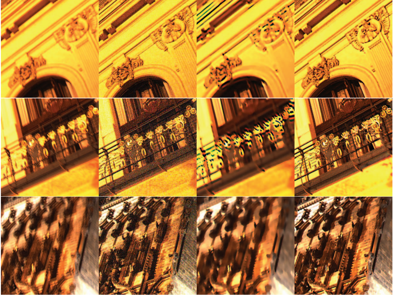
Fig. 3. Details of the image. From left to right – the blurred image, noisy image, the result of deconvolution by the kernel valid in the image center, our result.
