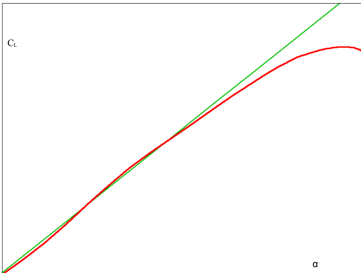
Illustration 1: Scheme of linear and nonlinear lifting line
