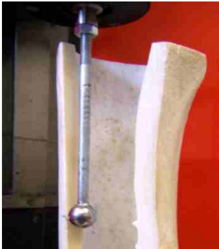
Fig. 4 The bone specimen and its shape measurement via contact probe on milling machine
