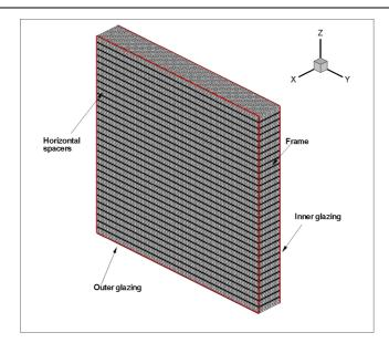
Figure 3. Mesh for the cavity with horizontal fins.
