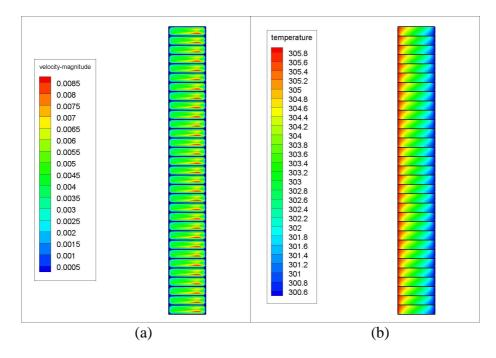
Figure 6. Velocity field, m/s (a) and temperature field, K (b) in the cavity with horizontal fins (Ra = 128000).
