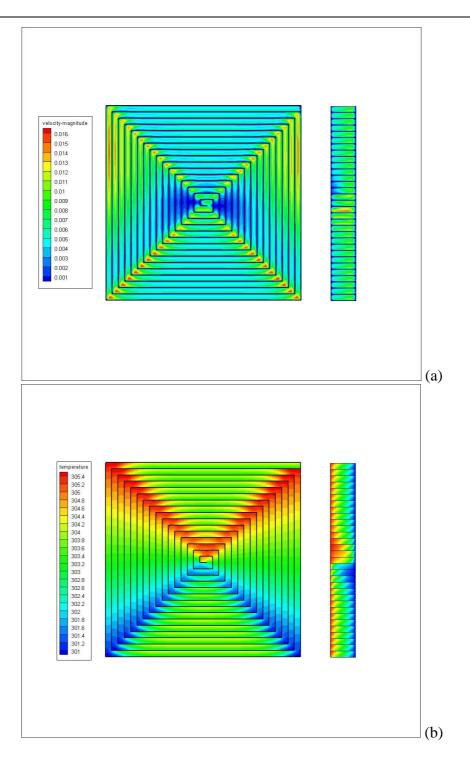
Figure 7. Velocity field, m/s (a) and temperature field, K (b) in the labyrinth-type cavity (Ra = 128000).
