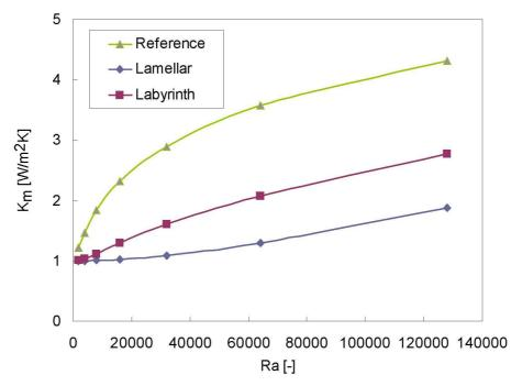
Figure 8. Global heat transfer coefficient for the three window geometries.
