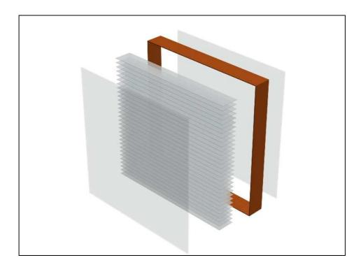
Figure 1. Structure of the double glazing window.
