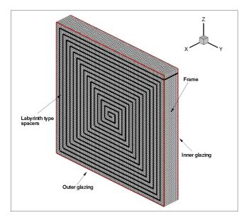
Figure 4. Mesh for the labyrinth cavity.
