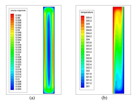
Figure 5. Velocity field, m/s (a) and temperature field, K (b) in the reference cavity (Ra = 128000).
