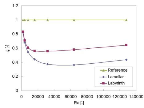
Figure 9. Dimensionless heat transfer coefficient of windows with different internal structure.
