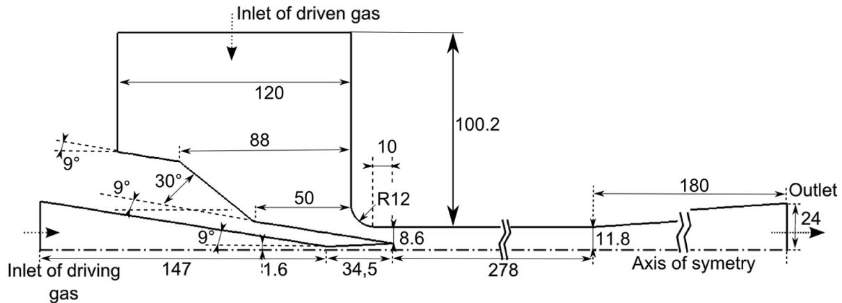
Figure 1: Model of the ejector (in millimeters)
