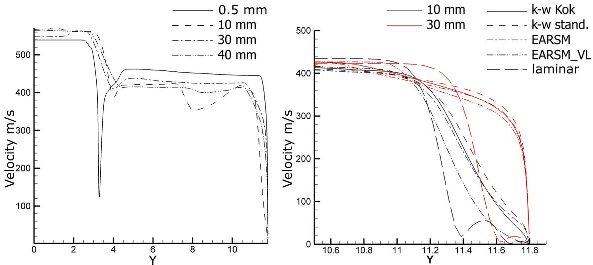
Figure 3: Velocity distribution across the mixing chamber at different points, on the left for  $k - \omega$  (Kok) and on the right for various models
