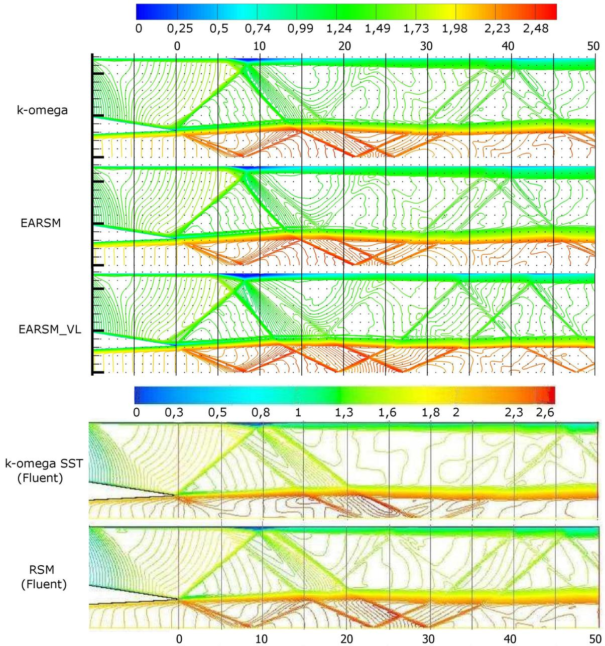
Figure 5: Mach number distribution (results with different models, Fluent [2])
