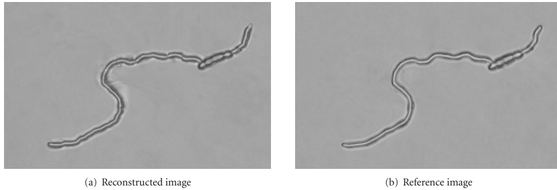
FIGURE 6: The specimen at a defined moment within in the interval between observations. The reconstructed image (a) was computed from the image in Figure 1(b) by means of a geometric transformation by thin-plate splines, mapping the control points in Figure 5(f) to their counterparts in Figure 5(d). The reference image (b) was acquired for the purpose of comparison at the corresponding stage of growth. The artificially generated image matches the authentic image almost perfectly, without unnatural deformations.
